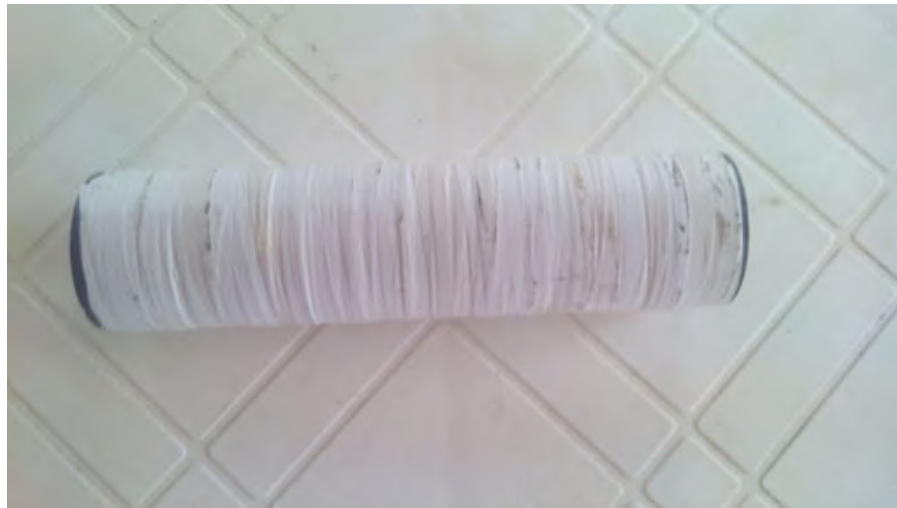
Fig. 36. A ferrite core made up of rings.
