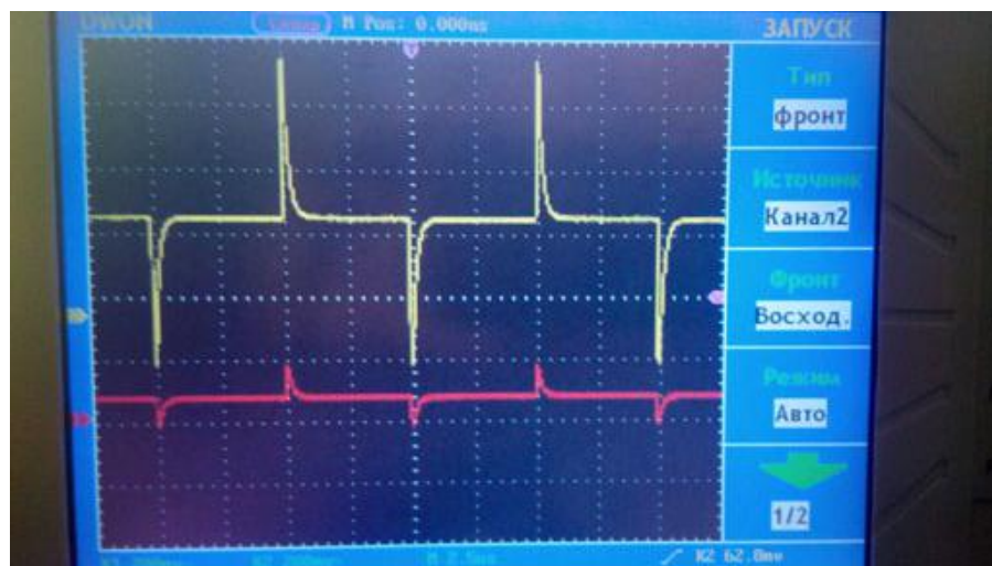
Fig. 40. Waveforms with a large-diameter inductor without ferrite, yellow - inductor, red "zero-transformer".
