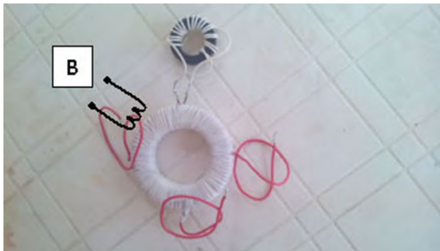
Fig. 51. The design of a "zero-transformer" similar to the Donald Smith version when wound on an annular core. Two
