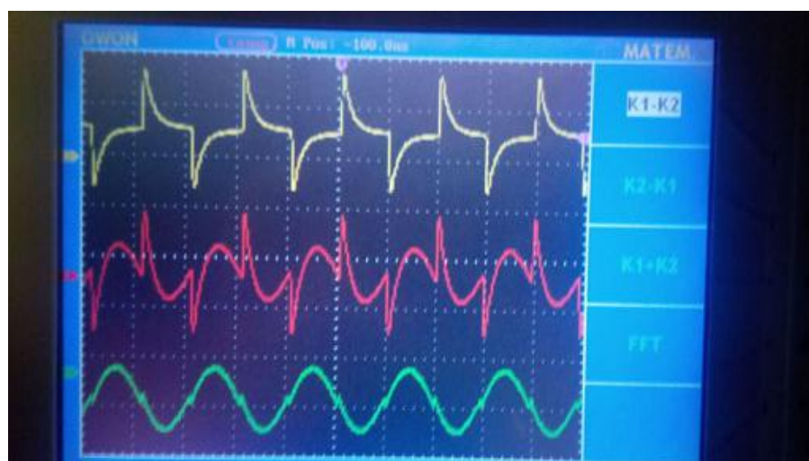
Fig. 55. Waveforms with pulsed excitation and resonance. Yellow - the input half, red - the entire coil, green - the second half.
