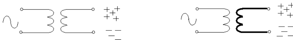
Fig. 4. Charge separation in the secondary winding of a conventional transformer at idle without energy consumption from the source.
