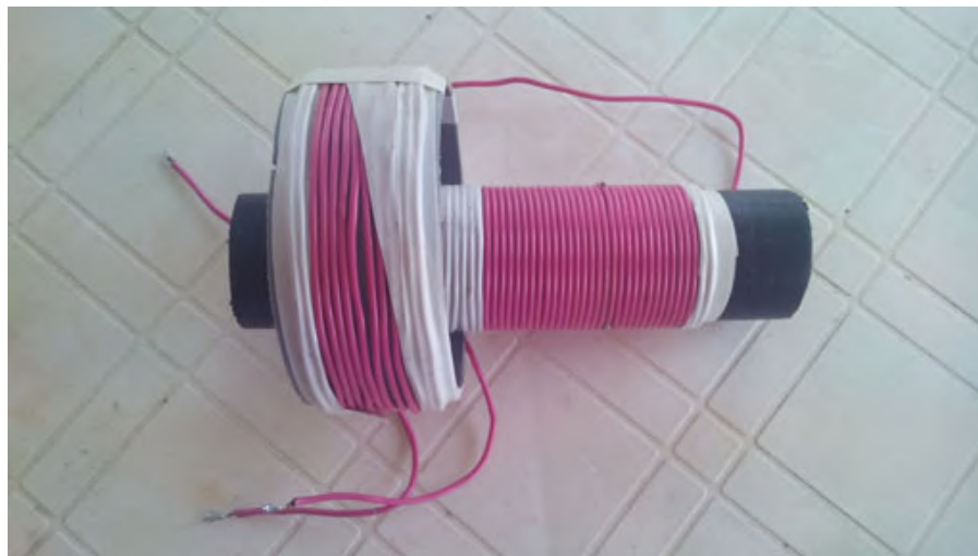
Fig. 39 "Zero-transformer" with a large-diameter inductor.
