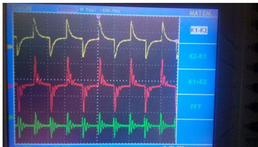
Fig. 54. An oscillogram with pulsed excitation without resonance. Yellow is the input half, red is the entire coil, green is the second half.
